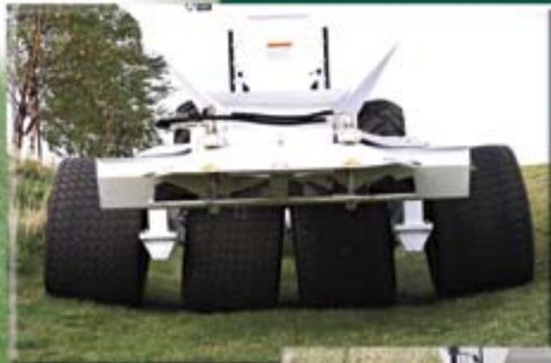
**DAKOTA walking beam axles have the lightest footprint in the industry.**
