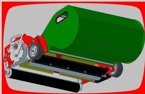
The counter rotating brush is very efficient in collecting any items from the green, including topdress material. It collects the cores from the GT 230 easily. Maredo is the only supplier who builds a counter rotating brush, using a gearbox with speed reduction. It is also ideal to brush in topdress material and brushing up the dense grass.
