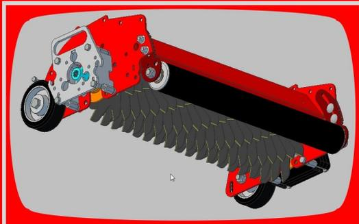
The main shaft of the regular slit verticutter is directly driven by the greensmower motor. It has tipped blades for outstanding lifetime. It does not collect the material, but leaves it on the surface, so it can dry. Next you can blow it off with the sand staying on the green.
