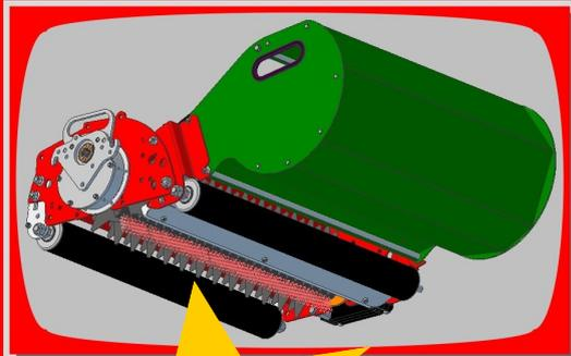
The Counter Rotating Random Verticutter is an innovative attachment. It looks like the GT180, but the (same) blades are mounted at an angle on the mainshaft.
