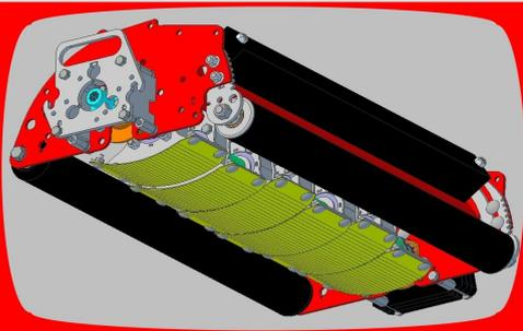
The GT300 works with 6 timed, curved shoe plates, who "walk" over the turf. The depth/ impact can be set by the front roller. Since the 6 sections are well timed, the impact is much more than with a roller. It pushes vertically down. A greenspeed increase of 30% in one pass is possible.
