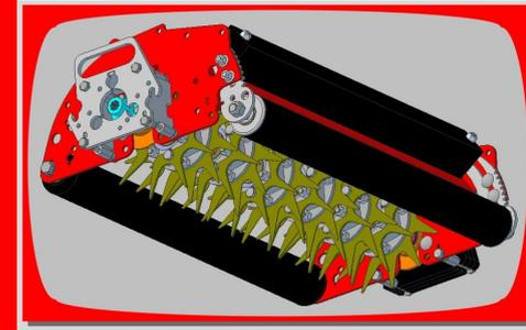
The 6 spike sections roll over the surface and are mounted on a driven camshaft, which add a vibration to the spikes. This vibration creates deep, nice holes. Other tools are available, like disks and thin slicer spikes.
