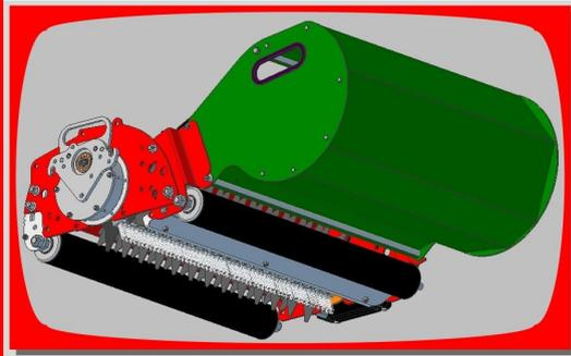
The Counter Rotating Slit Verticutter is a unique attachment for greensmowers, as the main shaft rotates against the drive direction at a reduced speed, due to the special gearbox. The reduced speed increases the torque on the shaft.
