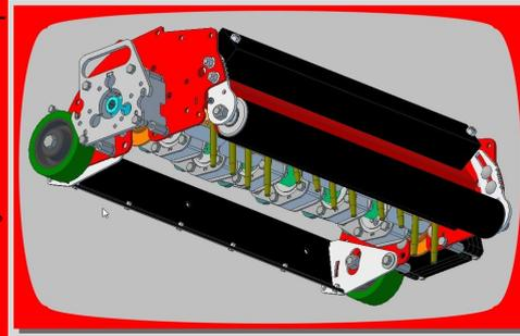
The Recipro Corer has become very popular as thatch remover on greens. It goes 25 mm (1") deep and leaves tiny holes, which are gone in 1-2 days. It is the quickest surface aerifier. The driving speed determines the hole spacing. **UPTO 4 MILLION HOLES PER HOUR !**
