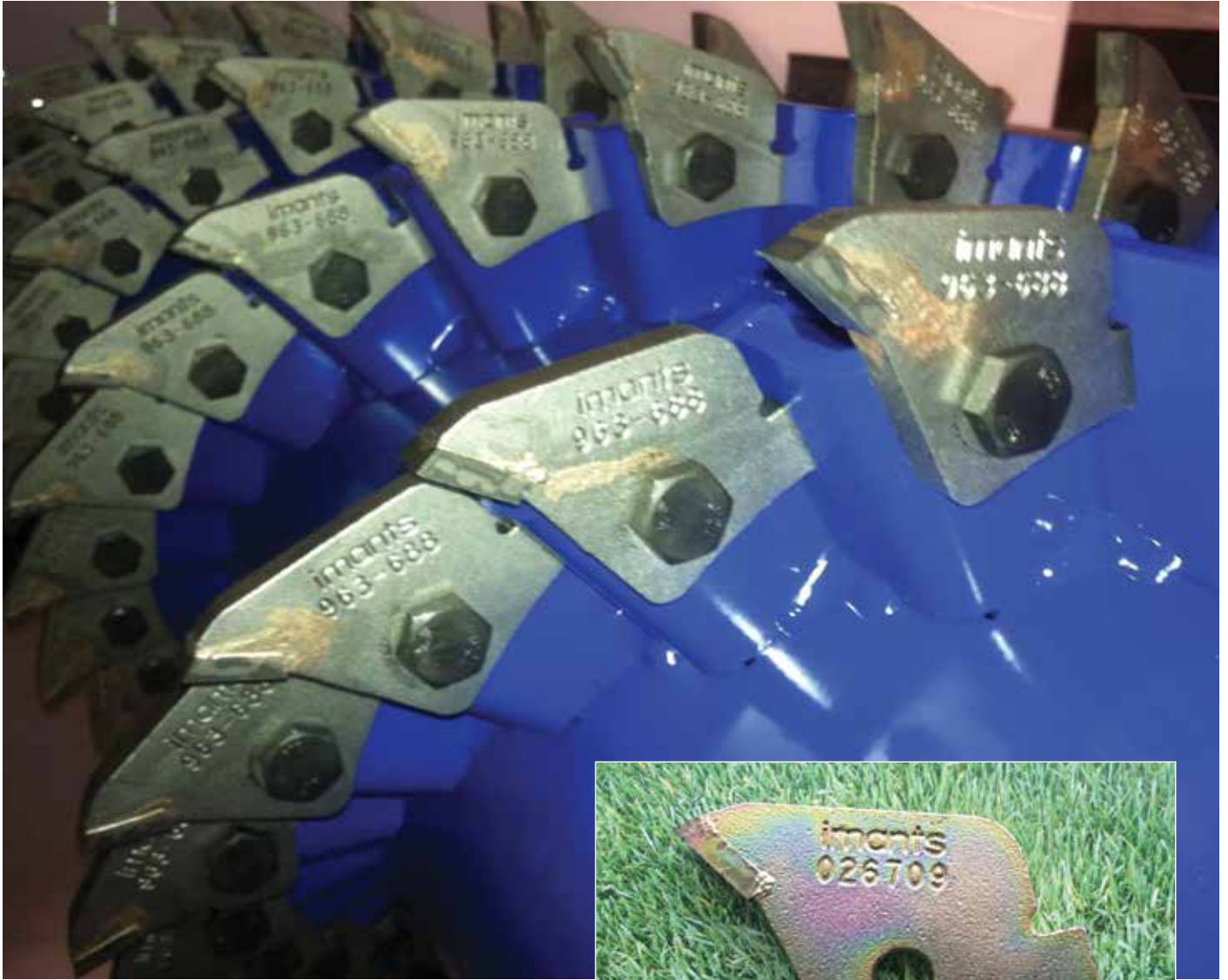
10mm tungsten tipped blades in 4 spiral Universe® rotor configuration
