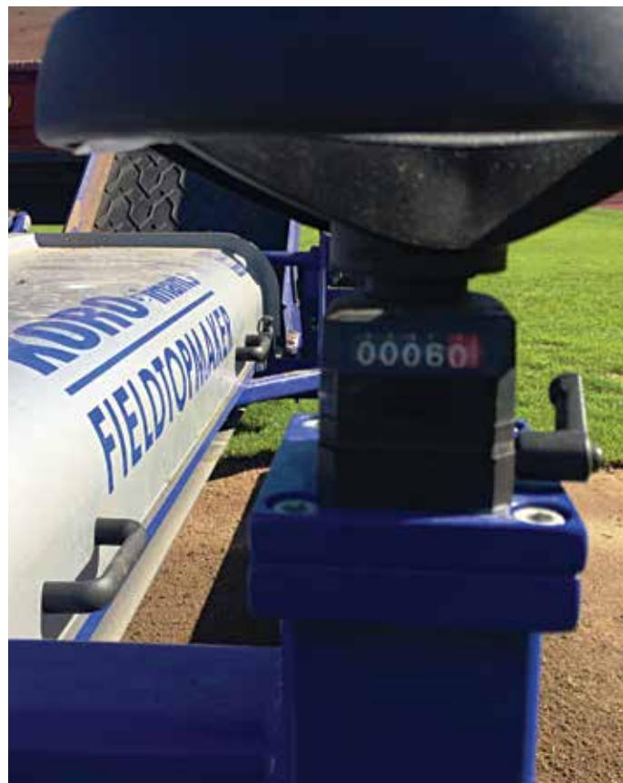
Depth setting is accurate to 0.1mm, via a digital display read out
