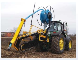
Trench widths are easily adaptable from 125mm to 400mm with digging booms for depths of up to 1.6m (63")
